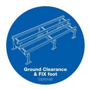
In some applications extra ground clearance is required, usually to give operators better access to the batteries. Our ground clearance solution can be added to the standard rack when there is a requirement for more space between ground and the stringers of the first tier: Alcad ground clearance is 300 mm.
